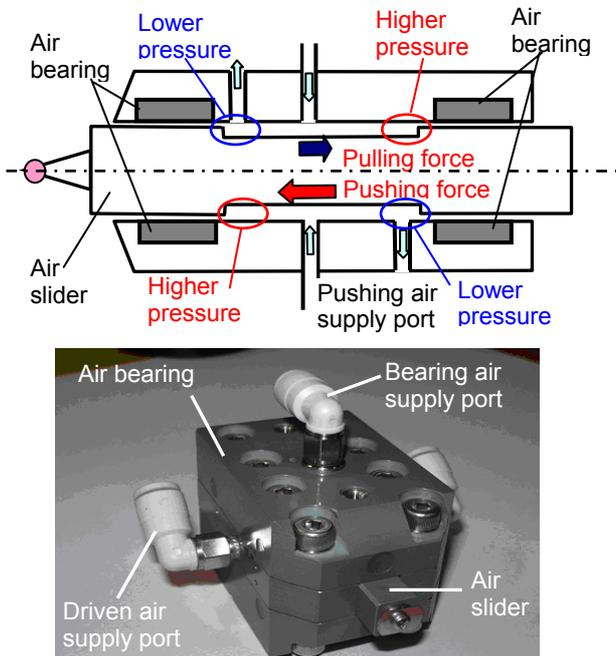
Figure 4: Schematic diagram and view of developed air slider for measurement unit.
