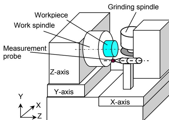
Figure 1: An example of conventional on-machine measurement system.
