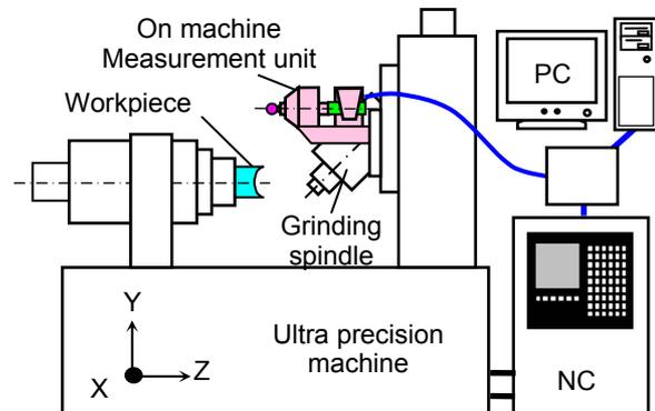
Figure 7: Schematic diagram of developed on-machine measurement system.
