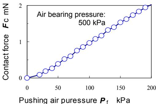
Figure 5: Relationship between supplied air pressure and generated contact force.
