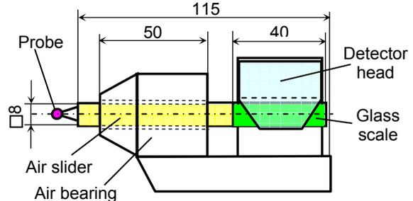
Figure 6: Measurement unit.
