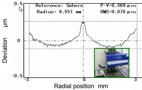
(a) Measured with conventional instrument
